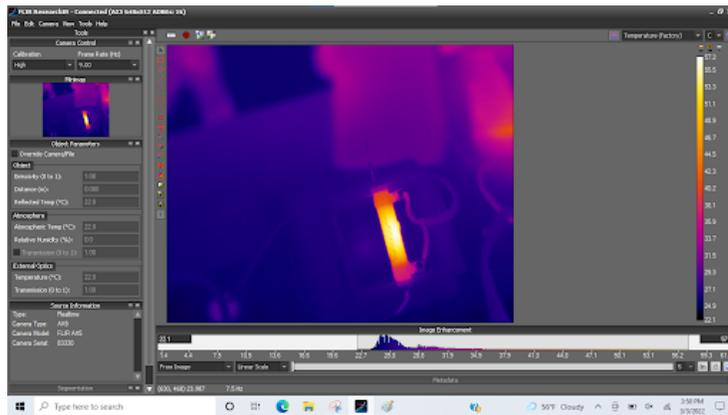
Figure 7: Temperature gradient of a resistor captured using the FLIR (forward-looking infrared camera)
