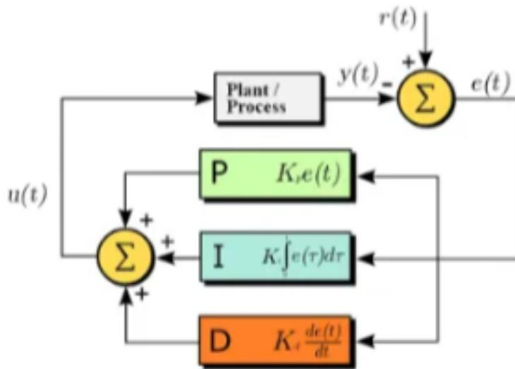
Figure 2: Block Diagram of the PID controller in a feedback loop
