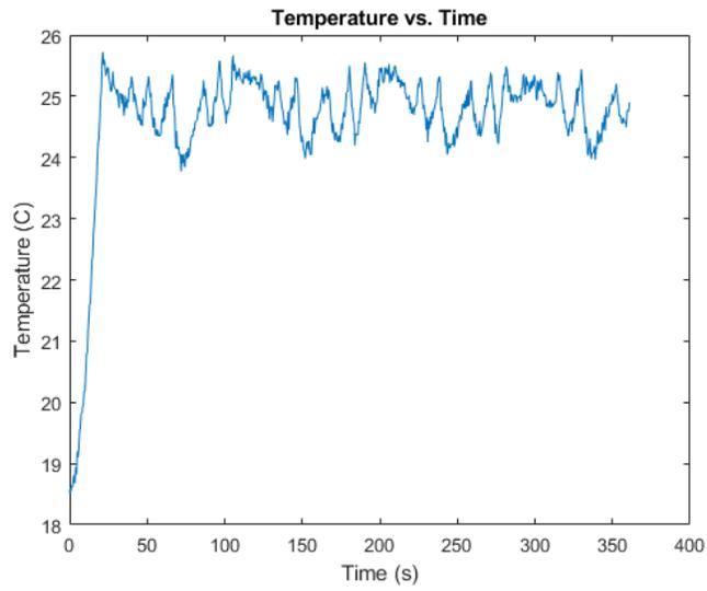
Figure 4: Temperature recorded with respect to time of the resistor
