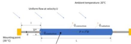
Figure 1: Cylindrical heated resistor in cross-flow
